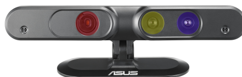
Fig. 22: Asus Xtion Live - with one infrared emitter (red), a rgb camera (yellow) and depth camera (blue) ©Asus
