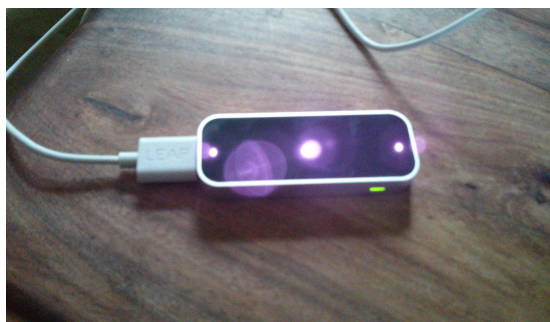
Fig. 23: LeapMotion device emits infrared light, which can be seen with a non-filtered camera
